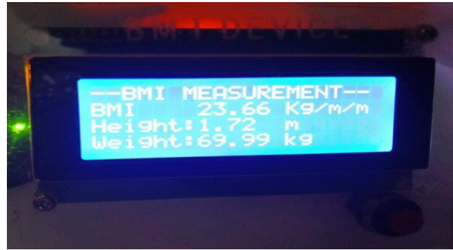
Figure 12: Device display the BMI, Height and Weight of the subject been measured.
