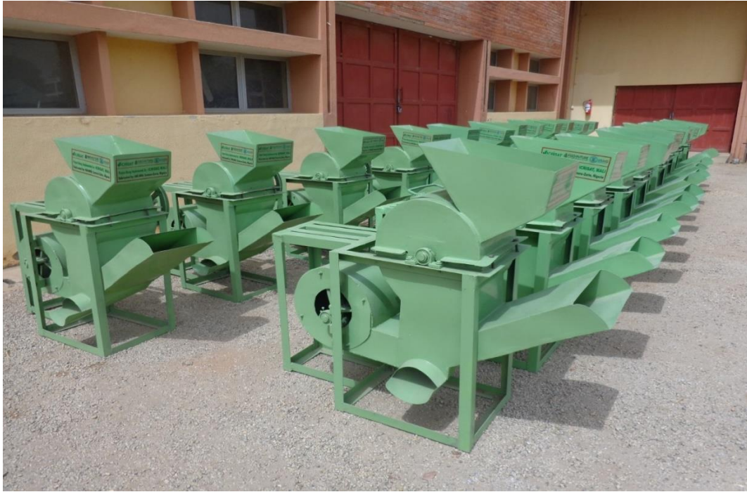
Groundnut/Cowpea Sheller -- For threshing of groundnut and cowpea.
