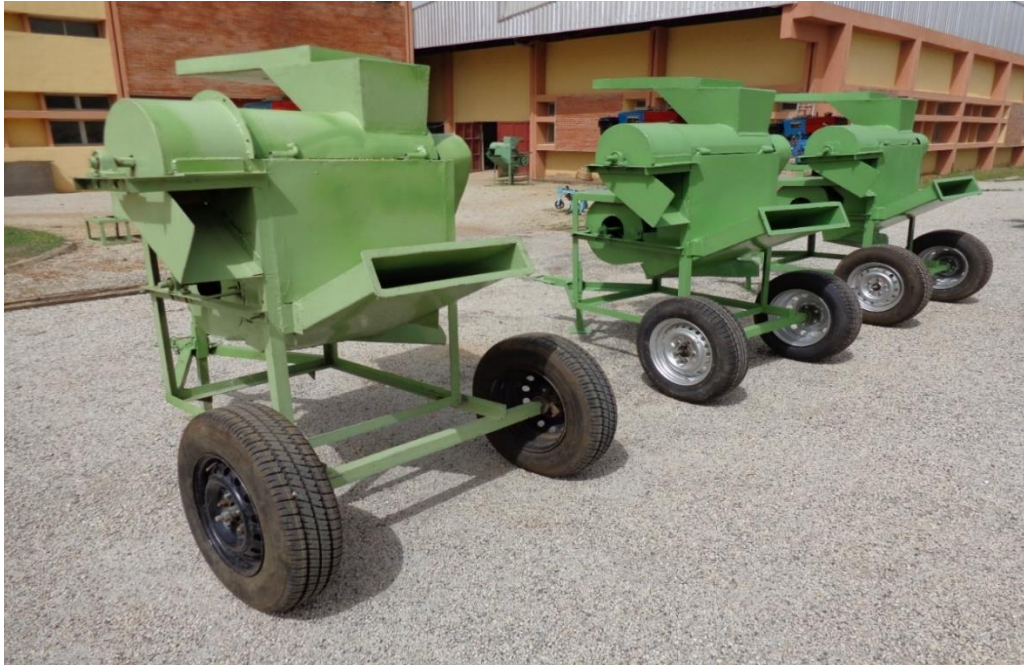
Maize Dehusker Sheller – For dehusking, shelling and cleaning of harvested corncob (maize) in one operation.
